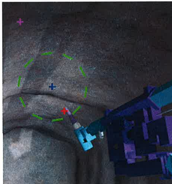
Figure 19: Automatic camera tracking keeps the nozzle(red) and hit point(pink)in view if possible .
