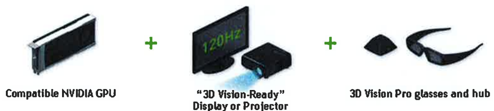
Figure 16: Equipment used for quad buffered stereoscopic 3D.
